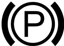
If equipped with an Electric Parking Brake (EPB), the EPB working indicator illuminates as the EPB is pulled up.
