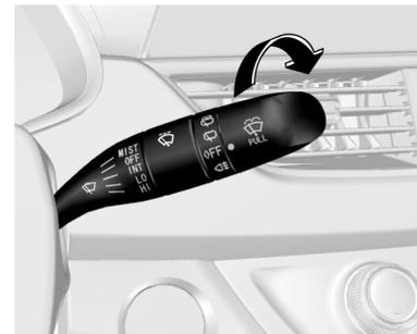
To use the rear windshield washer, turn the ignition switch to ON first and then turn the rear wiper and washer switch knob to
