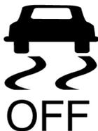
The StabiliTrak OFF warning light illuminates after the ignition is turned on and goes out several seconds later. This indicates that the warning light is working normally.
