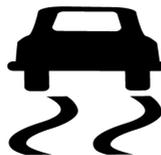
The warning light illuminates after the ignition is turned on and goes out several seconds later. This indicates that the warning light is working normally.
