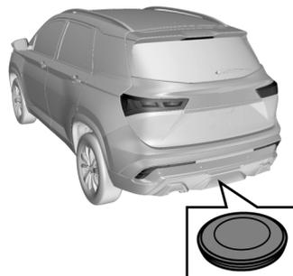
The spare tire for the 7-seat model is at the bottom of the vehicle rear floor.
