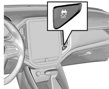
Press the ESC OFF switch after starting the vehicle, and the ESC OFF lamp on the instrument cluster illuminates and some ESC functions are disabled. Press the ESC switch again, and the ESC function is enabled again and the ESC OFF lamp on the instrument cluster goes out.
