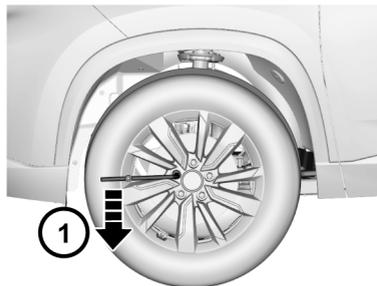
1. Take out the tools, jack and spare tire. Check and confirm that the tire on the diagonal is secured with wedges, blocks or stones.
