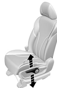
Turn the handle on the outer side of the seat upward or downward until the seat is adjusted to the desired height. Sit on the seat before adjustment; otherwise the adjustment device may be damaged.
