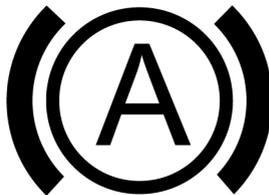
The automatic vehicle hold (AVH) working indicator illuminates after the ignition switch is turned on and it goes out several seconds later. This indicates that the indicator can
