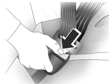
2. Put the latch plate in the buckle to secure the belt. Pull the shoulder belt to adjust the tightness of the hip belt.
