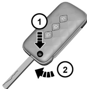
Press the release button (1), and the mechanical key (2) will pop up automatically.
