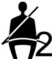
The seat belt warning lamp illuminates if the front passenger seat is occupied but the occupant does not fasten the seat belt properly after the ignition is turned on.
