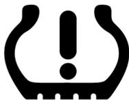
The tire pressure warning lamp illuminates after the ignition switch is turned on and goes out several seconds later. This indicates that the warning lamp is working normally.
