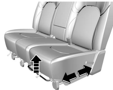
To adjust the seat forward or backward, pull up on the adjustment lever on the front lower part of the seat. Release the lever after the seat is adjusted to a proper position.
