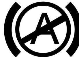
The automatic vehicle hold (AVH) fault warning lamp illuminates after the ignition switch is turned on and it goes out several
