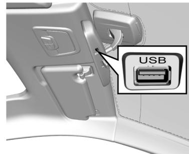
The driving recorder is at the bottom of the inside rearview mirror and can provide power for your driving recorder.
