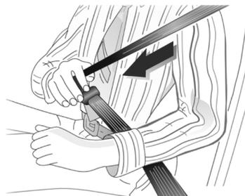
1. Pull out the seat belt from the retractor, and fasten it across the body without twisting.
