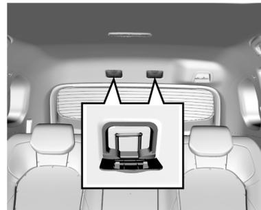
5. Connect the upper strap of the child seat to the corresponding fixing point of the vehicle. Refer to the child seat instructions for when and how to strain the upper strap. As shown in the figure, the ISOFIX upper fixing point is on the roof above the rear seat. Open the outer cover from the upper edge. The child seat upper fixing point of 7-seat models is on the back of the second row seat backrest.
