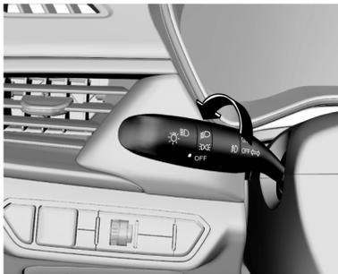
When the ignition switch is turned to ON, and the headlamp functions as a position lamp or in low beam, turn the ring button in the middle of the combination switch to ON (connected) to turn on the front fog
