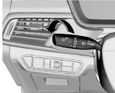
To switch the headlamp, tail lamp and parking lamp on or off, turn the end of the lamp control lever.
