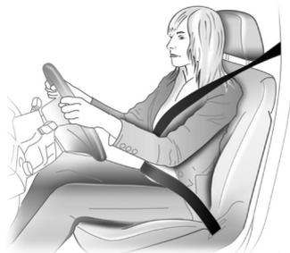
The seat belt is designed only for one passenger use. A passenger under 12 years old or under 150 cm high should not sit in the front passenger seat due to seat belt restrictions. Check all parts of the seat belt system for damage and abnormal function regularly.
