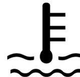
The engine coolant temperature warning light illuminates as you turn on the ignition, and it goes out several seconds later. It indicates that both the system and the indicator bulb are working normally.
