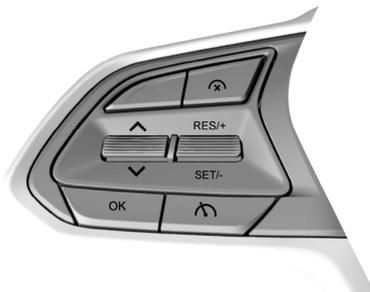
The cruise control buttons are on the steering wheel. When the cruise control system is started, the vehicle can run at the set speed. Press the brake pedal, and the function will be immediately disabled. Operating switches such as the parking brake and clutch can also disable the cruise control system. The system can be used at 3 (Third) , 4 (Fourth), 5 (Fifth) and 6 (Sixth) gears with the speed range of 40–120 km/h when the engine speed is lower than 4800 rpm.
