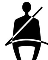
The seat belt warning lamp illuminates if the driver does not fasten the seat belt properly after the ignition is turned on.
