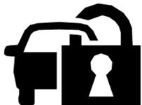
This indicator illuminates when the door is opened. It goes out after the engine is started. This indicates that the indicator is working normally.
