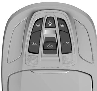
or : Press the button to open the left or right reading light, press it again to turn off.
