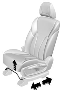
Pull upward on the adjustment lever on the front lower part of the seat to adjust the seat forward or backward. Release the lever after the seat is adjusted to a proper position.
