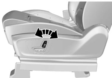
Turn the adjustment switch forward and backward. The backrest will be folded forward or unfolded backward. Release the switch when it is adjusted to a proper position.
