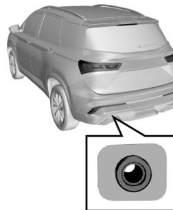
There is a hole cover on the left side of the rear bumper of the vehicle. Open it to access the fixing hole for hook installation.
