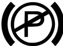
If equipped with an Electric Parking Brake (EPB), the EPB fault warning lamp illuminates after the ignition switch is turned on and it goes out several seconds later. This indicates that both the warning lamp and the EPB function module are working normally.
