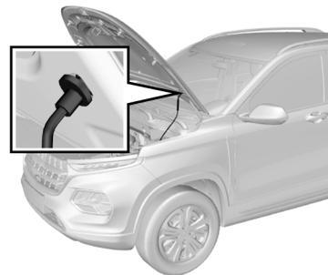
3. Separate the engine hood prop rod from the fixing clamp. Plug the free end of the prop rod in the slot.
