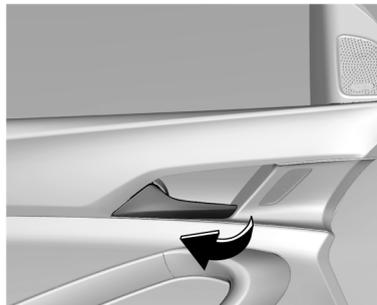
To open doors from inside or outside, unlock the doors first, and pull the external or internal door handles.
