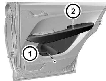
The door storage groove (1) and armrest (2) are on the inner side of the door panel.
