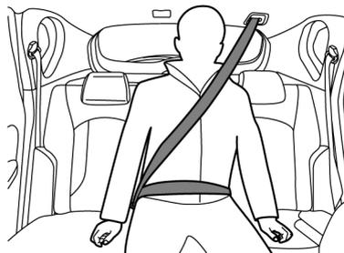
4. Make sure that the seat belt goes across the occupant's body without twisting.
