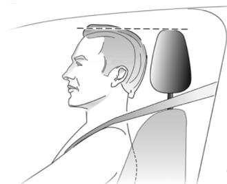
The middle position of the head restraint should be on the same horizontal line as the occupant's eyes. For tall persons, if the above point cannot be met, the head restraint should be adjusted to the highest position; for short persons, the head restraint should be adjusted to the lowest position.
