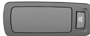
For second row seats, some models have two buttons on the roof for the reading light, press the button to turn on or off.
