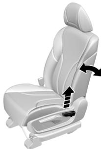
Pull up on the handle near the seat cushion; adjust the backrest inclination angle to a proper position; then, release the handle. Do not lean on the seat backrest while adjusting.
