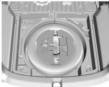
The spare tire, jack and tools are under the luggage compartment and can be seen after raising the luggage compartment floor.
