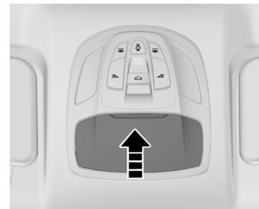
If equipped, there is covered storage for sunglasses in the overhead console. Press the outer cover and the console will open automatically. Close after use.
