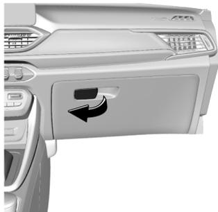
Pull the handle outward to open the glove box. To close, push and fasten the glove box door inward.
