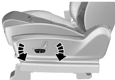
As shown in the figure, rotate the height adjustment switch on the outer side of the seat cushion, then release the switch after the seat is adjusted to the proper height.
